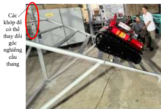
Figure 4.2: Experimental staircase with joints manufactured to change the angle of inclination
