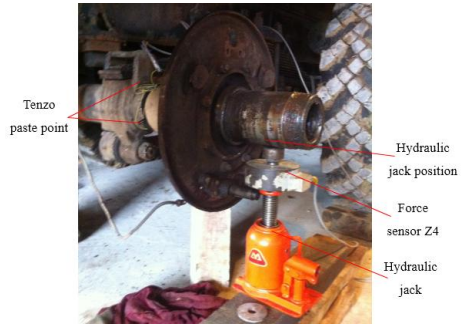
Figure 4.11: Calibration of normal jet measurement value
