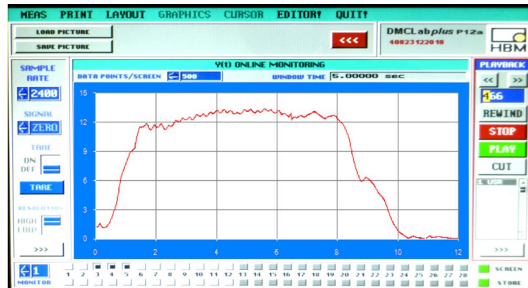
Figure 4.4. Result of measuring the horizontal inclination angle of boat
