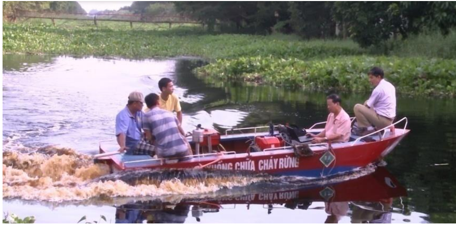
Figure 4.3. Experiment of measuring the horizontal inclination angle when the boat rotates with the highest steering angle
