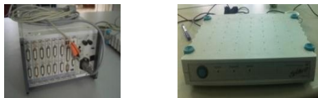
Fig 4.5 DMC plus and Spider8 musurement equipment
