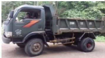
Fig 4.10 Three tons small truck experimental
